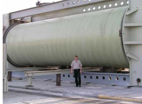
**Figure 3** – 78 inch Diameter FRP pipe/joint pressure test w/shear load at 362 psi
