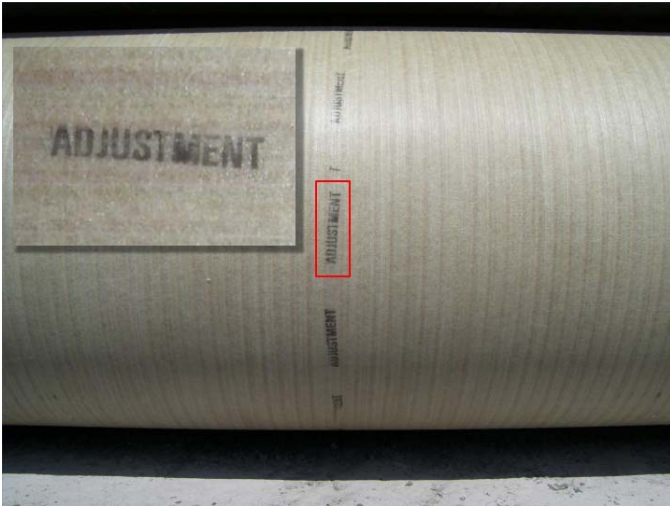
Check Spigot Tolerances; Adjustment Pipe Preferred
